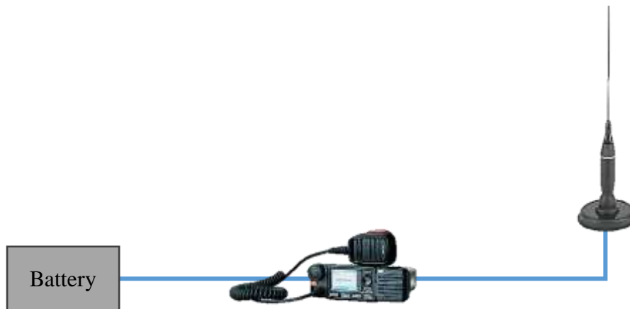
Figure F. Typical Single Line Diagram for Mobile Base Radio Station
